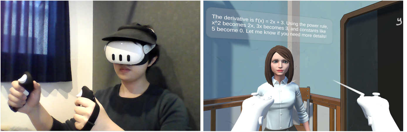
Fig. 1. The left image shows a user operating the Quest 3, while the right image displays the first-person view in VR Math Bridge, featuring the AI assistant and a virtual blackboard.
